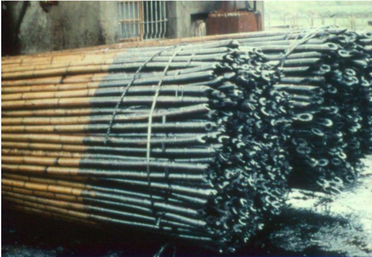
Pressure treatment with creosote caused environmental damage
