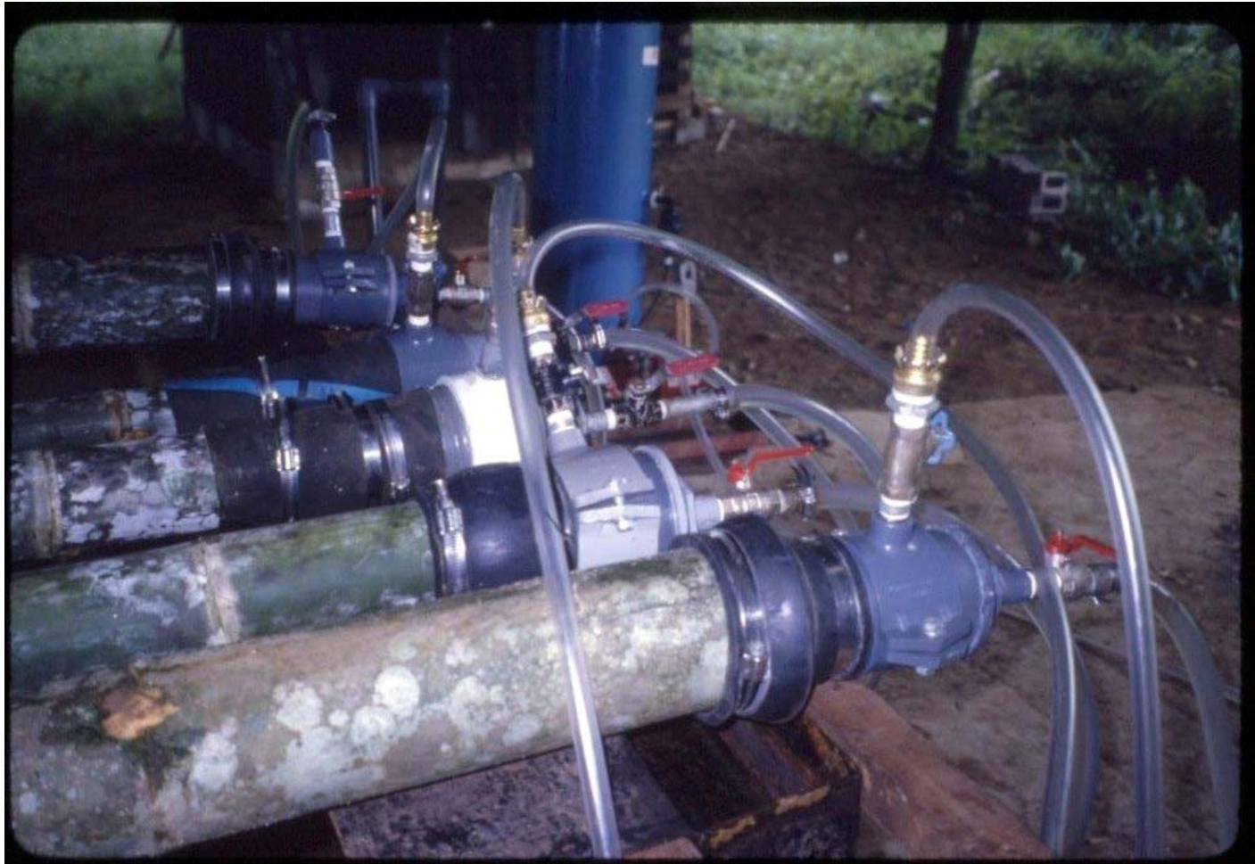
A valve at the pressure cap releases air to let preservative pressed in
