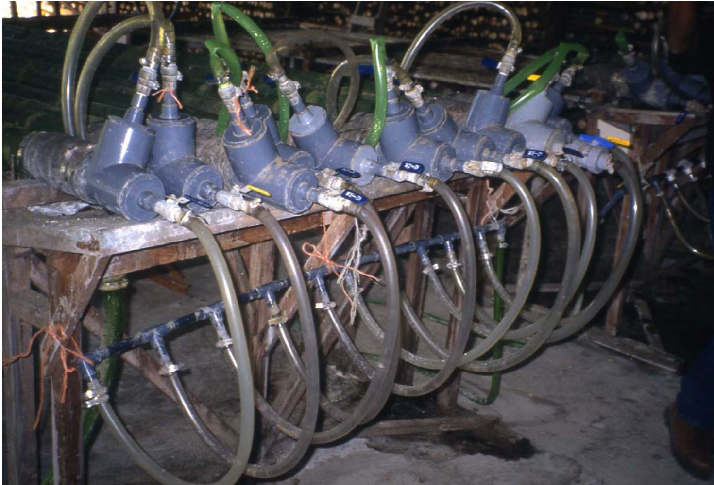
FUNBAMBU: Sap replacement treatment for constructions, Photo J. Janssen
