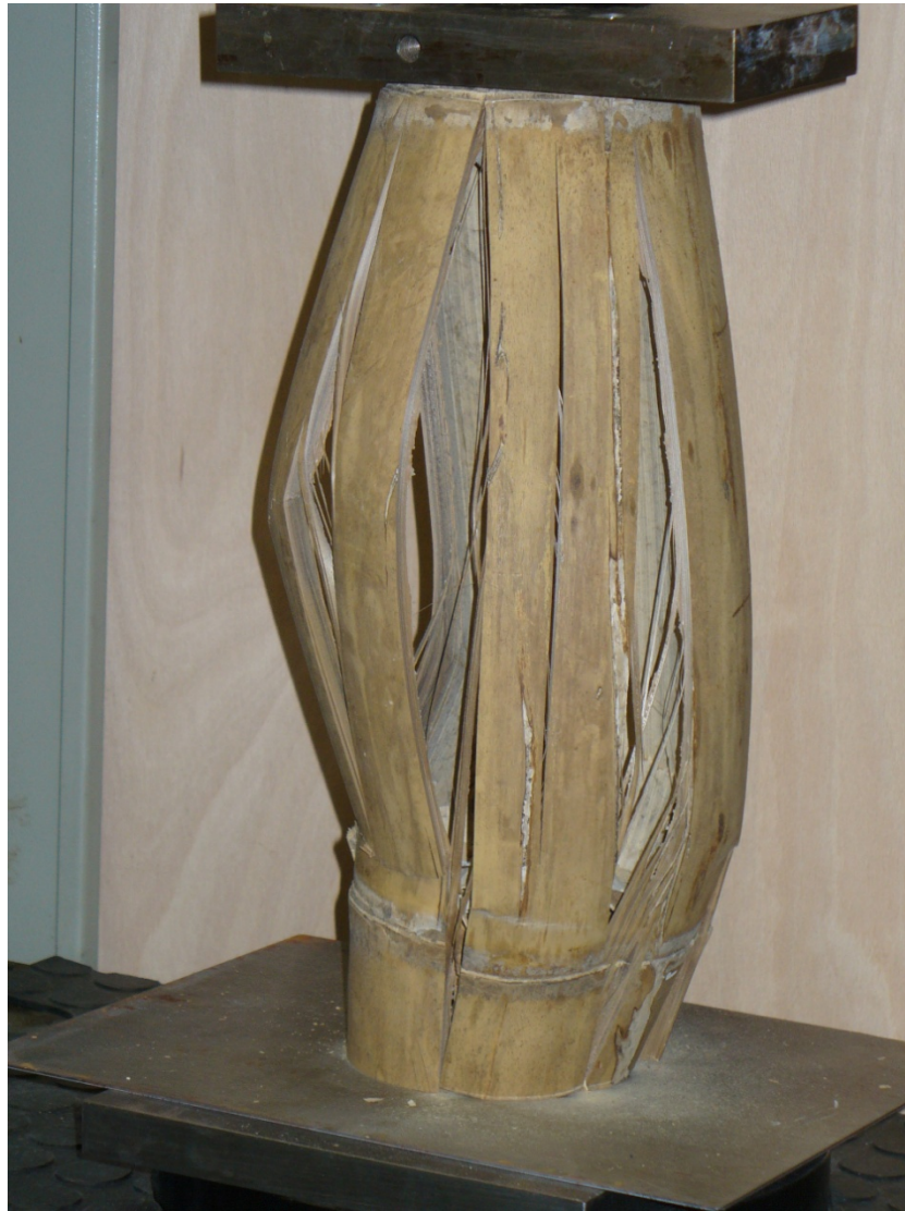
Rupture of an internode at 16 to.
