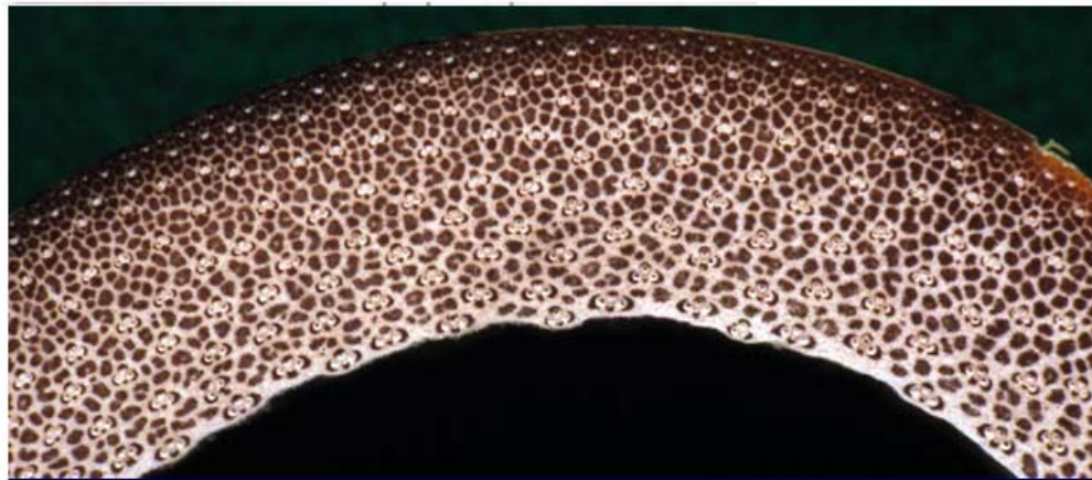
Vertical Soak Diffusion System (VSD) for bamboo preservation
