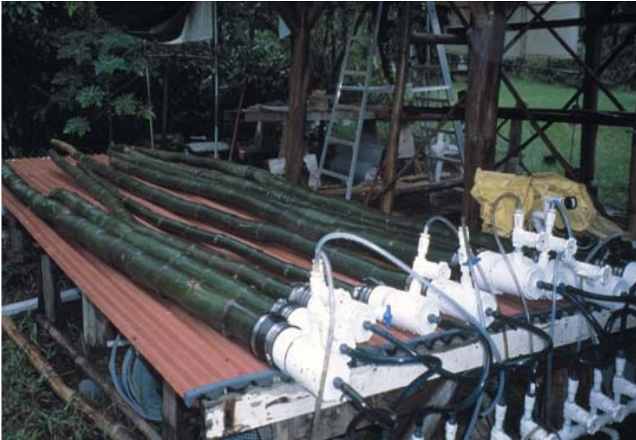
Bamboo culms treated by the sap replacement system, EBF, Bali
