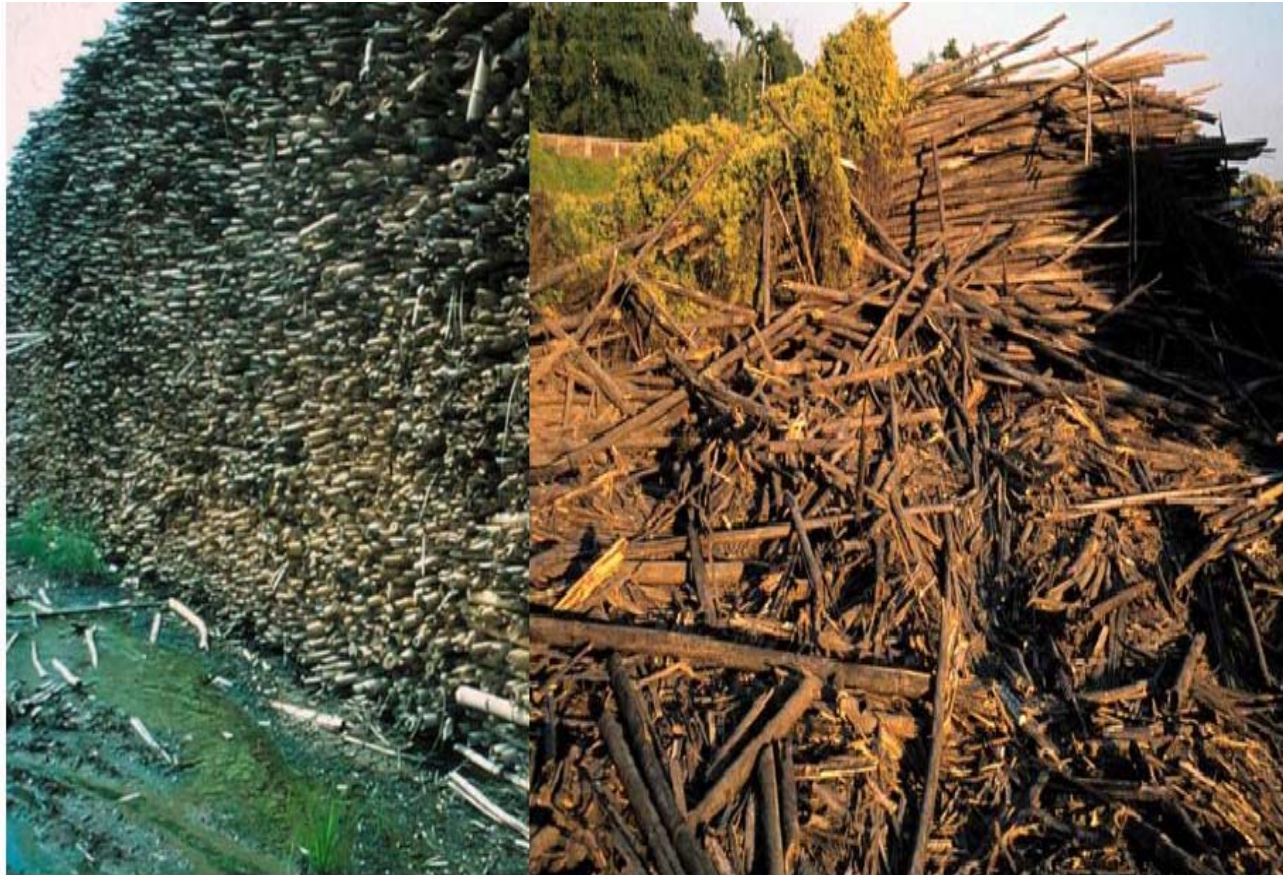
Bamboo storage at a pulp mill, degraded after 2 years
