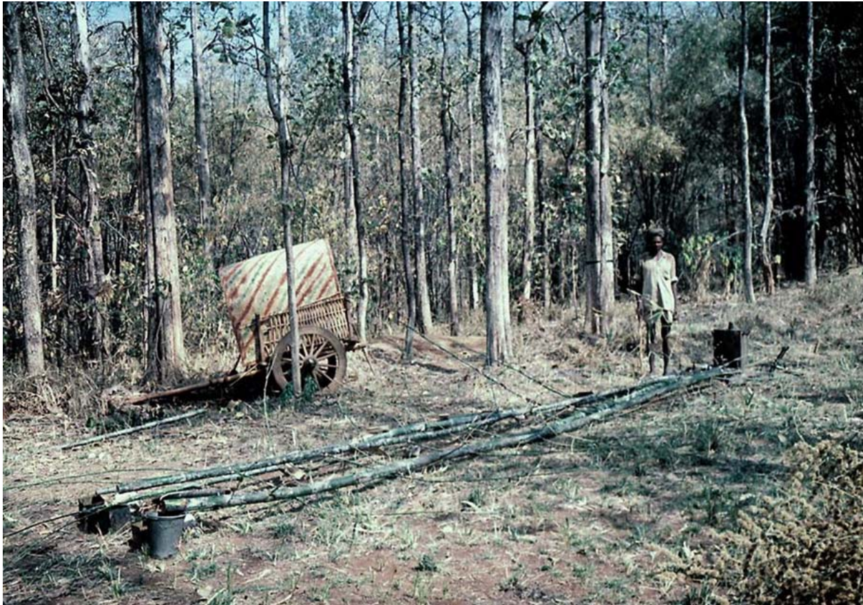
Trials to treat bamboo culms directly in the forest with the sap-replacement system
