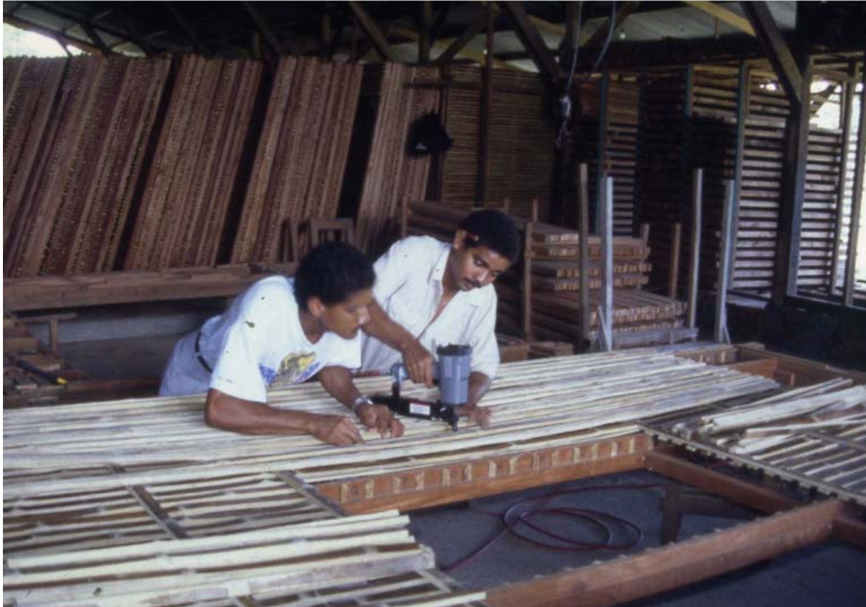
FUNBAMBu; Production of prefab. panels. Photo J.Jansen
